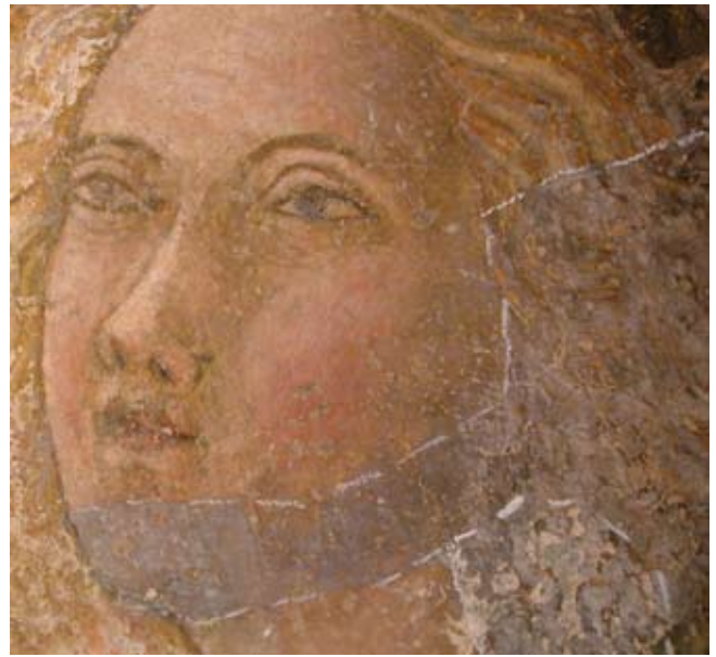
Laser cleaning where pigments are present is still an open issue: here laser cleaning of deteriorated frescoes was demonstrated at the S. Maria della Scala in Siena using the photo-thermal effect called 'laser spallation'
