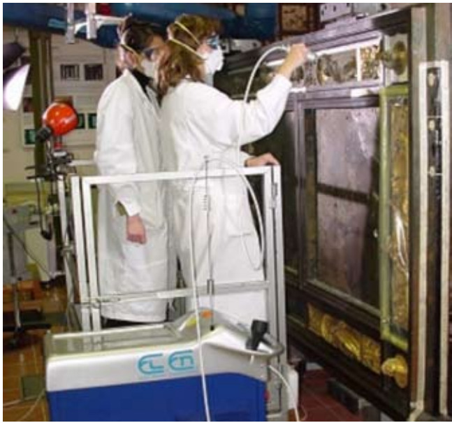
Laser cleaning of gilded bronze is today a well-established technique: the first demonstration has been the cleaning of the renaissance masterpiece by Lorenzo Ghiberti Gates of Paradise
