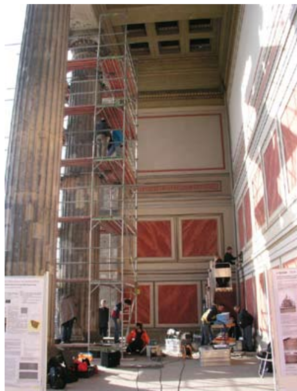
Different investigation methods performed (radar, impact-echo, ultrasound) – © FP5 ONSITEFORMASONRY project
