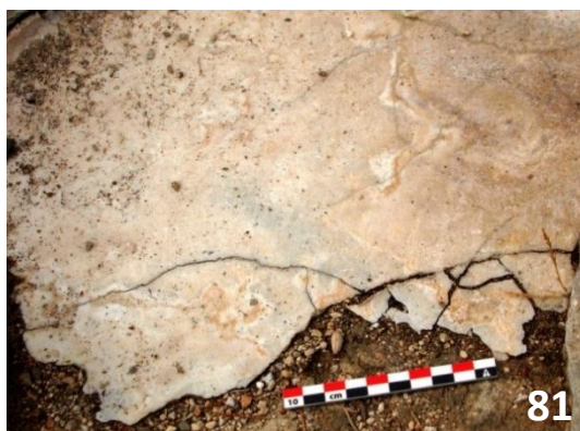
Figures 81, 82: Crack & Deformation; Secondary mineral gypsum from the “King’s Megaron” showing a network of thin cracks. Cracks due to mechanical stress from the “North Entrance”.
