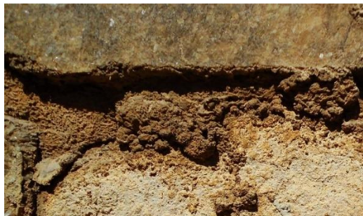
Figure 86: Erosion; Typical formation of microkarst cavities on the surface of secondary gypsum from Knossos. Dissolution pits, grooves and runnels, collectively called karren.
