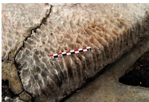
Figure 85: Disintegration; Loss of cohesion between gypsum crystal aggregates leading to crumbling. Selenite block located near the “West Magazines”, Knossos Palace.
