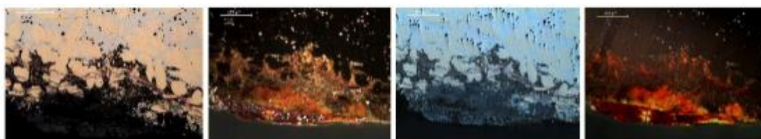
Figure 44: Metallic surface observed in different modes: Brightfield, Darkfield, Interference contrast and polarized light.
