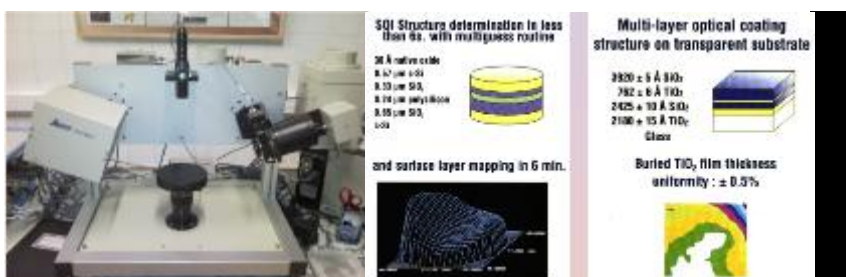
Figure 48: Jobin Yvon ellipsometer and example of surface layer mapping of silicon over insulator and determination of a multi-layer structure.
