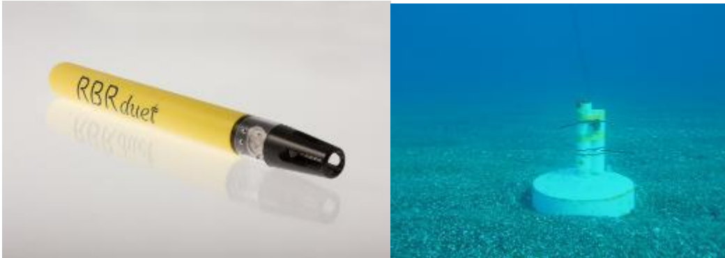
Figure 26: RBRduet sensor (left) and example of an installation base (right).
