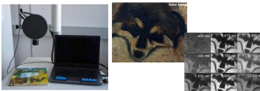
Figure 28: (left) The IRIS-II system, (center) the object under study and (right) the recorded spectral images at different spectral bands.
