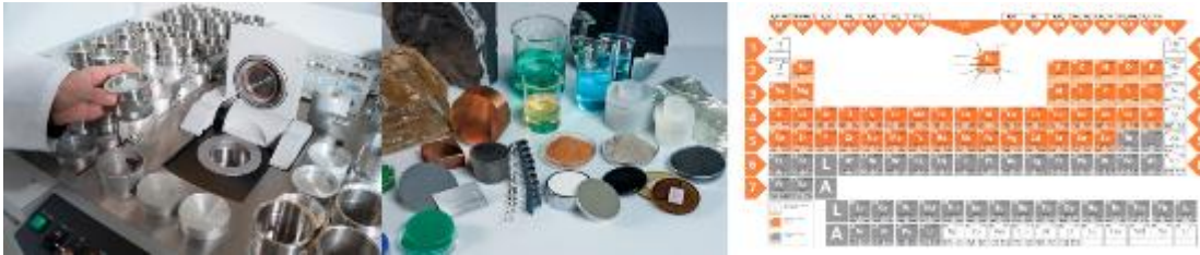
Figure 37: XRF (PANalytical) apparatus and different typologies of samples that can be analysed for elemental chemical analysis
