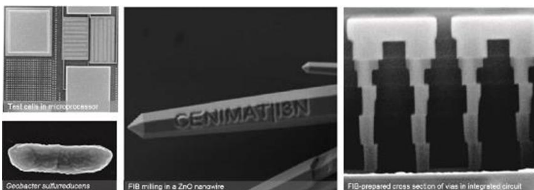
Figure 32: SEM FIB images of a microprocessor, bacteria, ZnO nanowire and nano-circuits prepared by FIB
