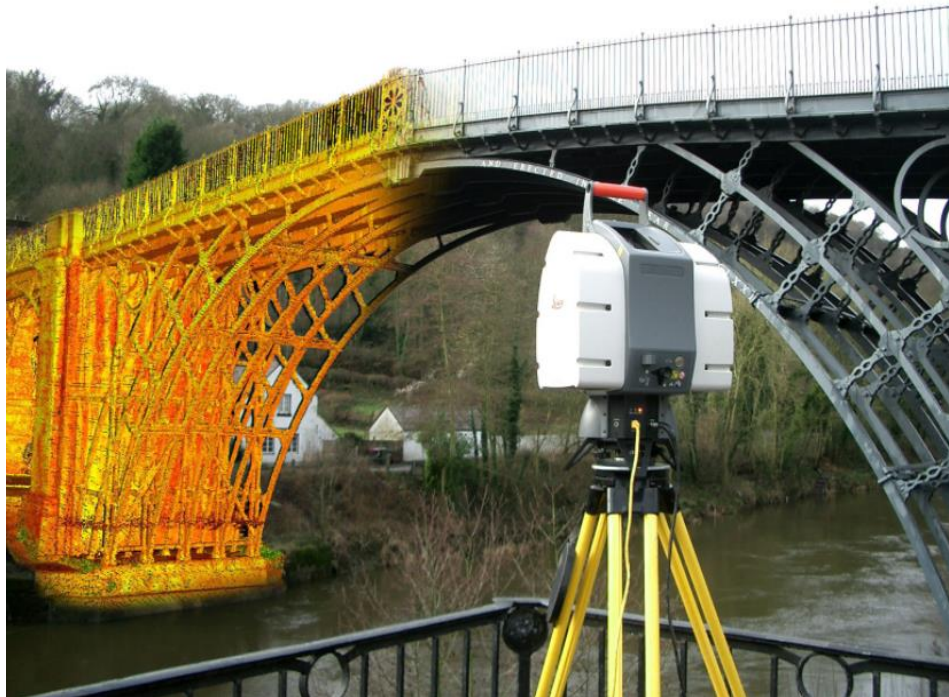
Figure 41: example of a TLS relief and of a points cloud
