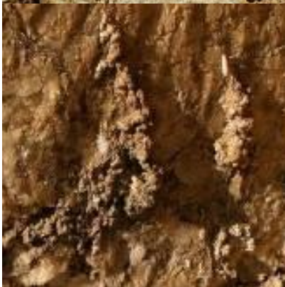
Figure 22: Recrystallized gypsum accumulations on the surface of selenite. Coarse crystalline gypsum (selenite) from the West Court, Palace of Knossos.
