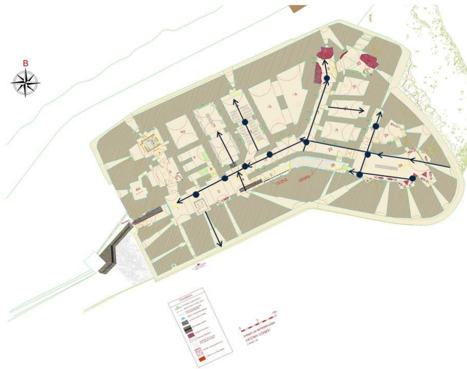
Figure 52: An attempt to show the GPR activities (vaulted constructions, fractures, existence of moisture) on the plan.
