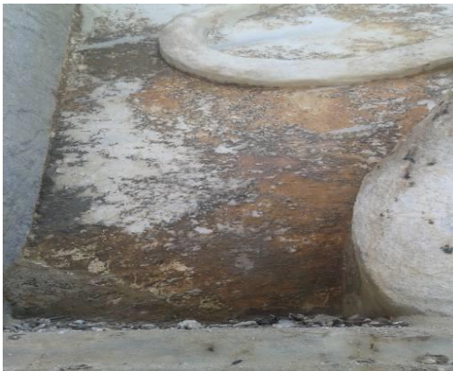
Figure 50: Black-brown hard crust on lion's surface (SE side).
