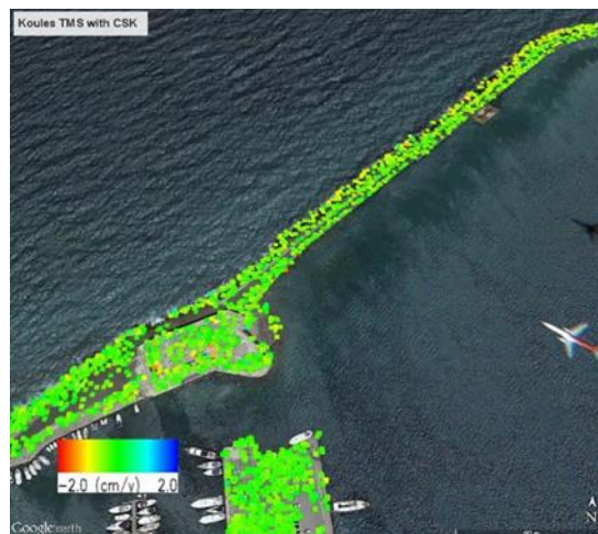
Figure 65: TMS preliminary results on Koules achieved by descending CSK passes
