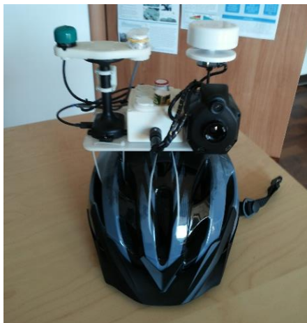
Figure 42: Miniaturized environmental payload mounted over a helmet.
