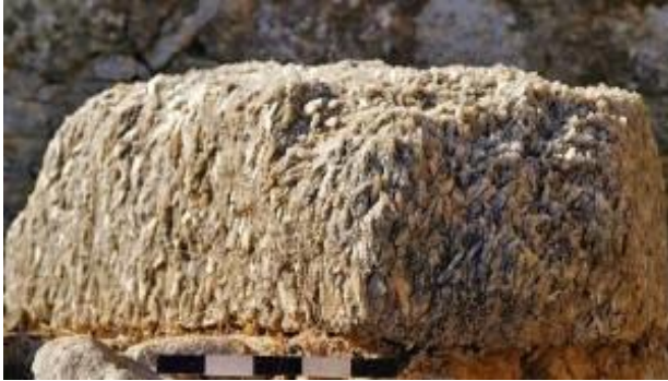
Figure 17: Loss of cohesion between gypsum crystal aggregates leading to crumbling. Selenite block located near the west magazines, Palace of Knossos.
