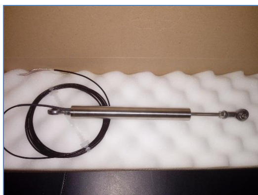
Figure 35 - LVDT used for the static monitoring of Consoli Palace
