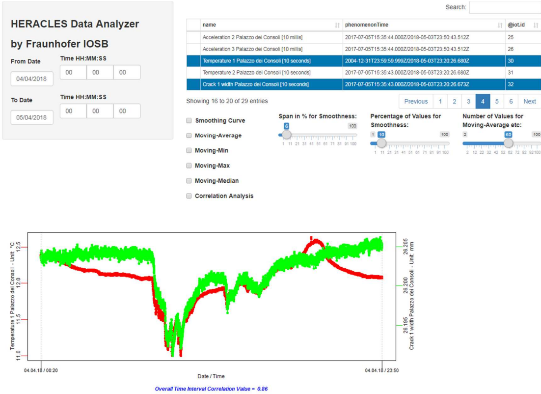
R based HERACLES Data Correlation Analyzer illustrating Gubbio Palace temperature and crack displacement values during a selected time interval on 4 th of May 2018
