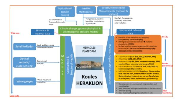
The following sensors/analysis were installed and carried on:
