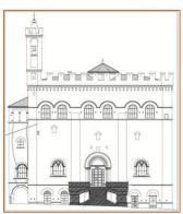
and vertical scans. It can be verified that the determination of the facade dimensions and proportions is based on the "golden rectangle", a geometric figure whose proportional laws are multiples of the golden ratio, concept always appreciated in classical antiquity, rediscovered in the late Middle Ages and propagated later during Renaissance.
