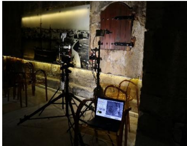
Figure 3. The Multispectral imaging setup for measurement of the efflorescence extent.
